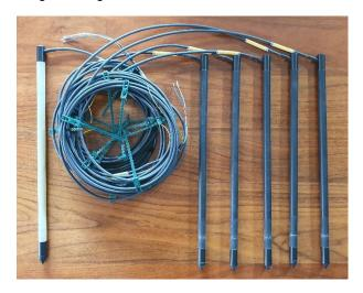
Our soil Redox probes and reference electrodes have probes bodies that are made from glass-fiber reinforced epoxy (GRE). GRE has a high mechanical strength and a very good chemical resistance. This makes it an ideal material for our probes, which are used under extreme environmental and climatological conditions, ranging from agricultural soils to estuarine sediments, and from tropical to arctic temperatures.
